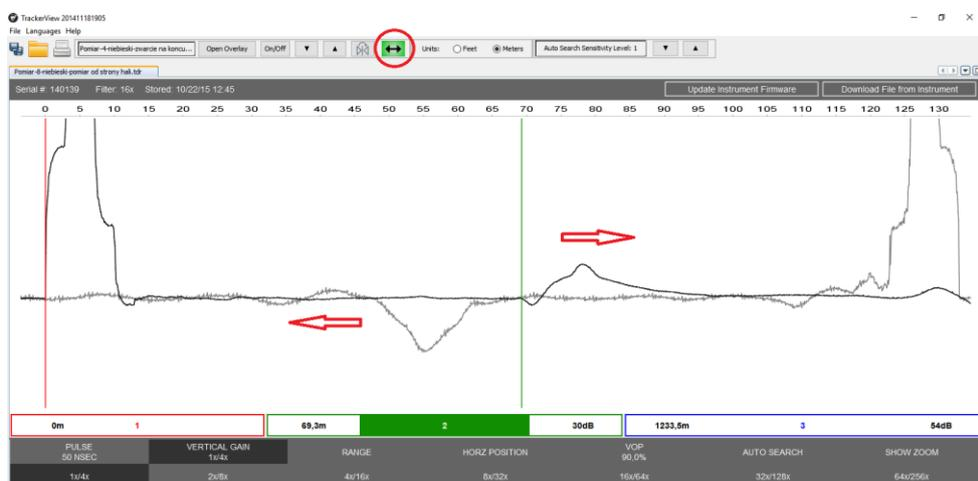
**Note:** Both features: „Mirror Horizontal” and „Drag Overlay Waveform” are active only when you overlay waveforms (compare two graphs on the screen).
