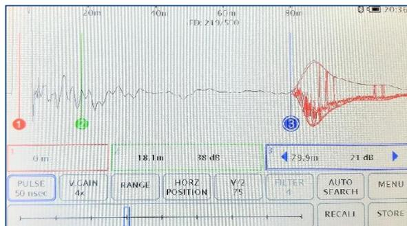
**NOTE:** The Tracker Pro TDR enables you to record intermittent faults on the cable only on individual pulse widths such as 2 nsec, 5 nsec, 20 nsec, 50 nsec, 100 nsec, 300ns, 500 nsec, 1000ns and 2000ns.
