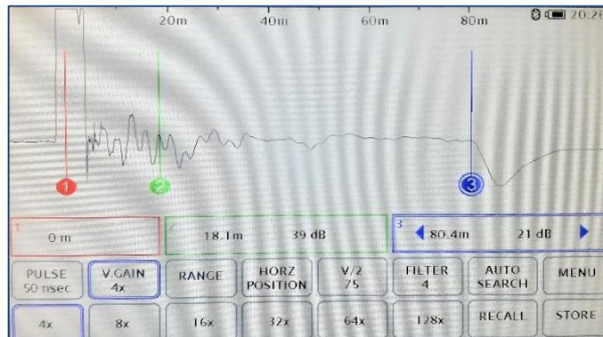
**Joint** A typical picture of a joint along the cable, the green cursor is on the joint (an upward reflection immediately followed by a downward reflection). The blue cursor marks the end of the cable. The below picture comes from the TrackerView application for PC.
